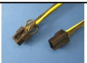
PCIE-86FM-XX PCI-E 8-pin Female to PCI-E 6-pin Male
