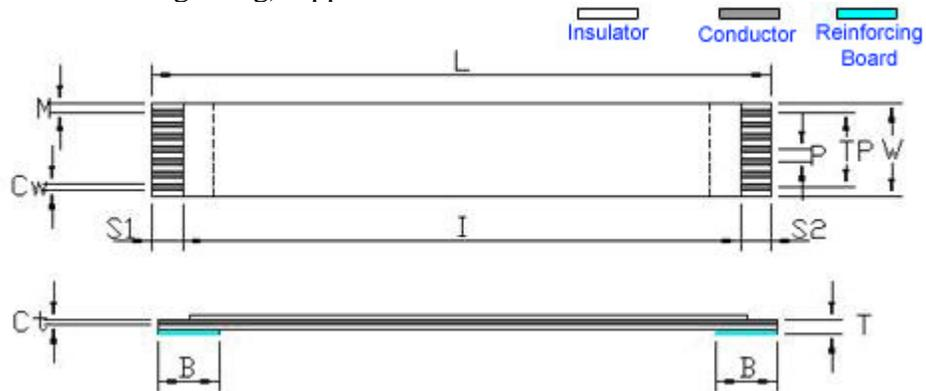
Light weight and ultra thin, FFC is ideal for tight spaces and an excellent alternative to standard IDC ribbon cable assemblies where bulk and rigidity would be an issue.
